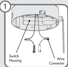
If your fan does not have pin connectors on the wires coming from the switch housing, install the wiring harness provided. Using the provided wire connectors connect the white wire from the fan to the white wire from the wire harness and connect the black or blue wire from the fan to the black wire from the wire harness.
